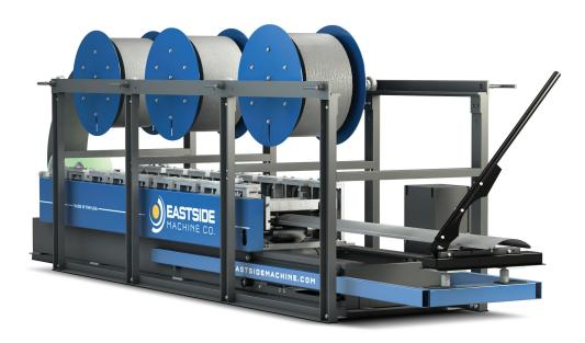
The EM 8 Log portable seamless siding machines are robust and the profile is extremely realistic. This user-friendly machine is designed, engineered and made in the USA. The patented roll-forming profile is unique and looks great on the wall. Eastside's siding machines feature our original self-contained embossing system, which applies a natural wood grain texture to steel coil.
