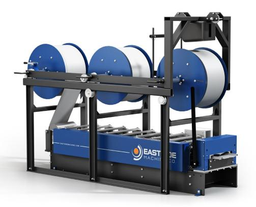
Eastside's portable EM 10 Snap Lock Roofing Machine is designed specifically for residential and light commercial applications. Its 9 3/4-inch rib-to-rib panel width gives it a look that belongs on homes, while other commercial roofing machines create panels that are not quite aesthetically correct.
